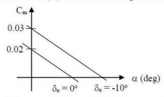
Based on the result presented in the figure above, the value of elevator control power  $(C_{m\delta e})$  in per radian will be (in three decimal place).
